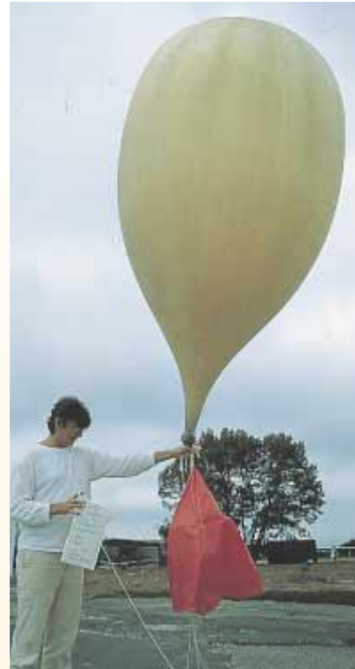
FIGURE 1 The radiosonde with parachute and balloon.
