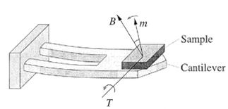
If material posses anisotropy, sample produces torque on lever,  $T = \vec{M} \times \vec{B} \propto B^2$ .
