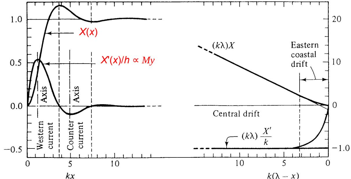
$$X_n(x) = \underbrace{-A e^{-kx/2} \cos\left(\frac{\sqrt{3}}{2} kx + \frac{\sqrt{3}}{2k\lambda} - \frac{\pi}{6}\right)}_{W} + \underbrace{1 - \frac{1}{k\lambda}(kx - e^{-k(\lambda-x)} - 1)}_{C} \equiv X(x) \quad \underbrace{\qquad}_{E}$$
