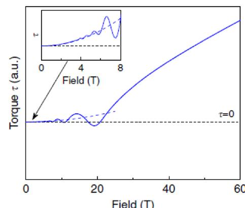
Massive fermion – no anomaly in magnetic response near quantum limit and no sign reversal in the torque.
