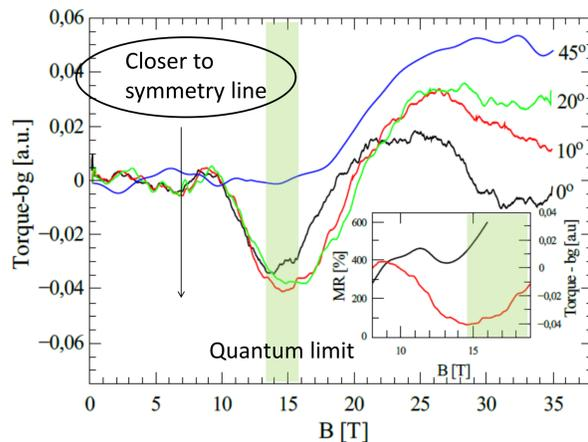
By entering the quantum limit the torque anomaly appears. Anomaly and change in torque slope is highly suppressed at 45°.
