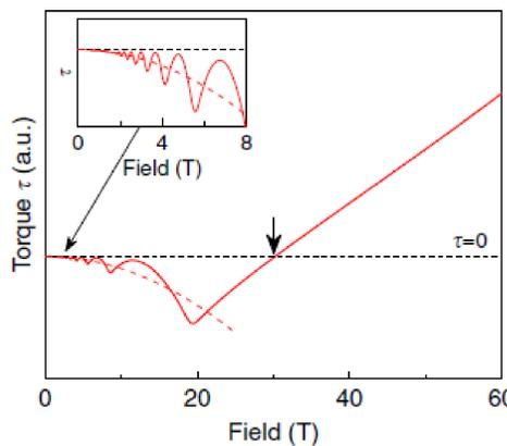
Weyl – a change from diamagnetic to paramagnetic response leading to the torque reversal.
