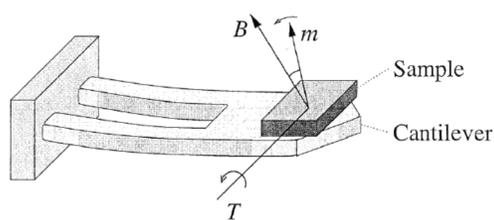
If material possesses anisotropy, sample produces torque on lever,  $T = \vec{M} \times \vec{B} \propto B^2$ .
