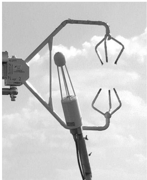
**Fig. 6.14** Sonic anemometer USA-1 with inclined paths and omni-directional construction (published with kind permission of © METEK GmbH, Elmshorn, All rights reserved)
