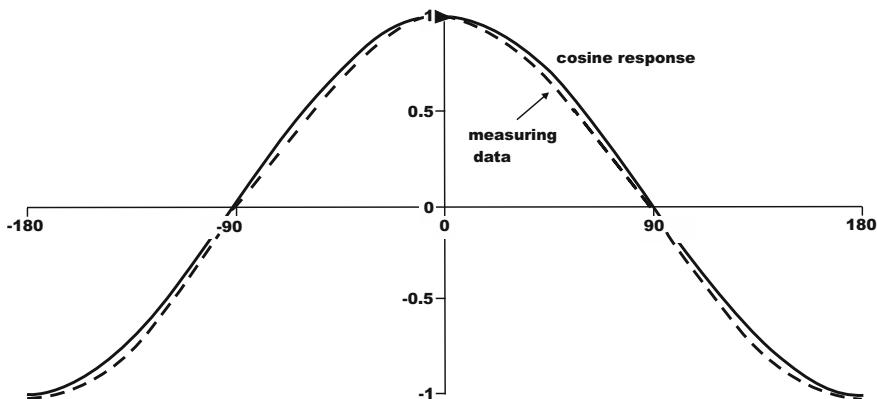
**Fig. 6.10** Cosine response of a propeller anemometer
