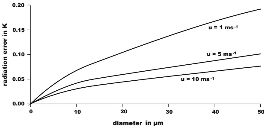
**Fig. 6.16** Radiation error of thin platinum wires for  $K_{\downarrow} = 800 \text{ W m}^{-2}$  and  $\alpha = 0.5$  (adapted from Foken 1979, with kind permission of © Wiley-VCH, Weinheim 1979, All rights reserved)
