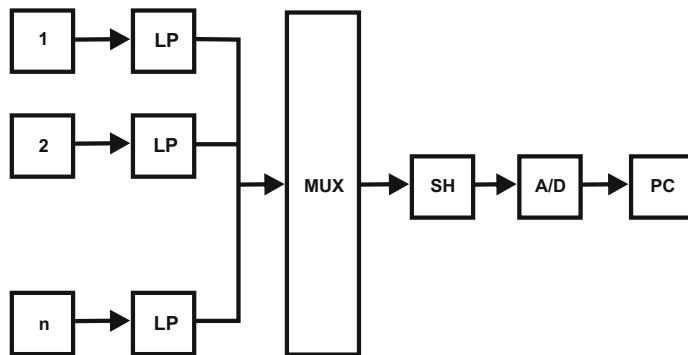
**Fig. 6.1** Basic circuit of a data sampling system with 1 to n signals, low passes (LP), multiplexer (MUX), sample and hold circuit (SH), analogue-digital converter (A/D), all integrated in a modern logger and a data collection computer (PC) or storage medium
