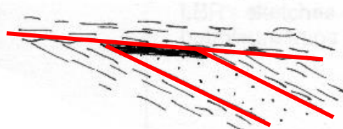
Trap at an unconformity (A surface of erosion buried by later layers)
