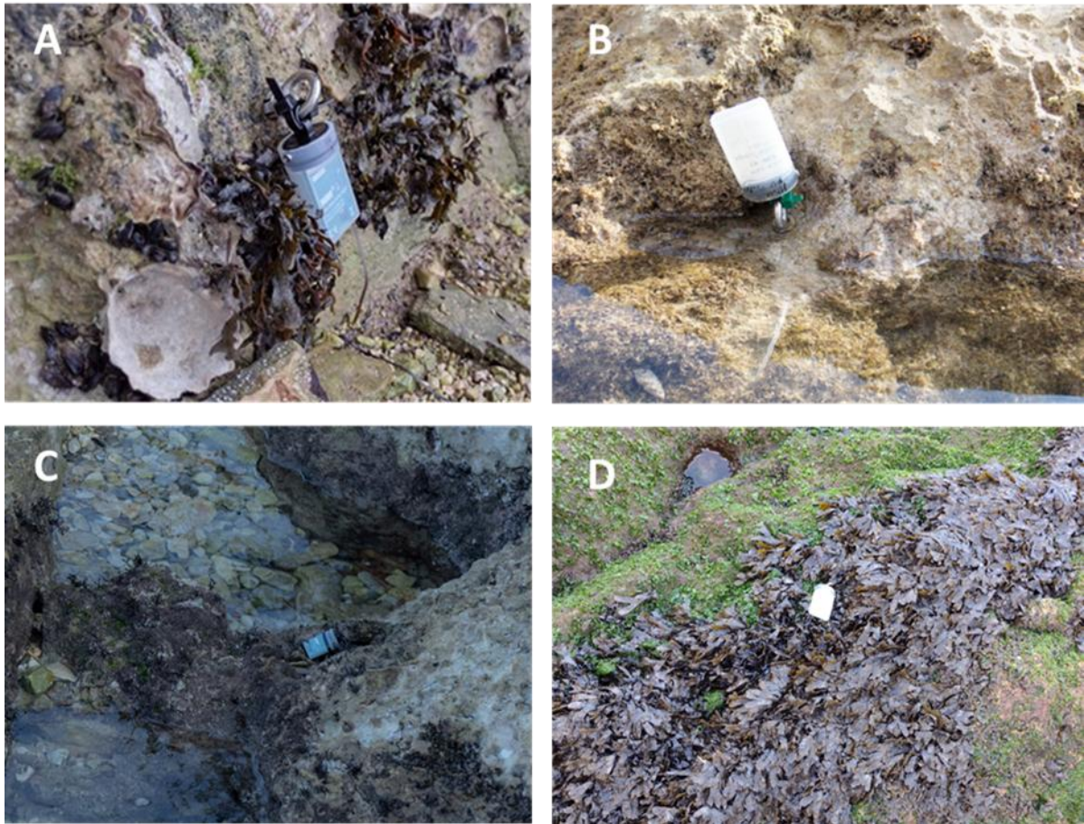
Figure 9. HOBO Pendant® Temperature/Light 64K data loggers mounted within the monitored Fucus virsoides communities for temperature and light measurements in 4 most representative stands: Lanterna (A), Hotel Parentium (B), Bijela uvala (C), and Blaz cove (D).
