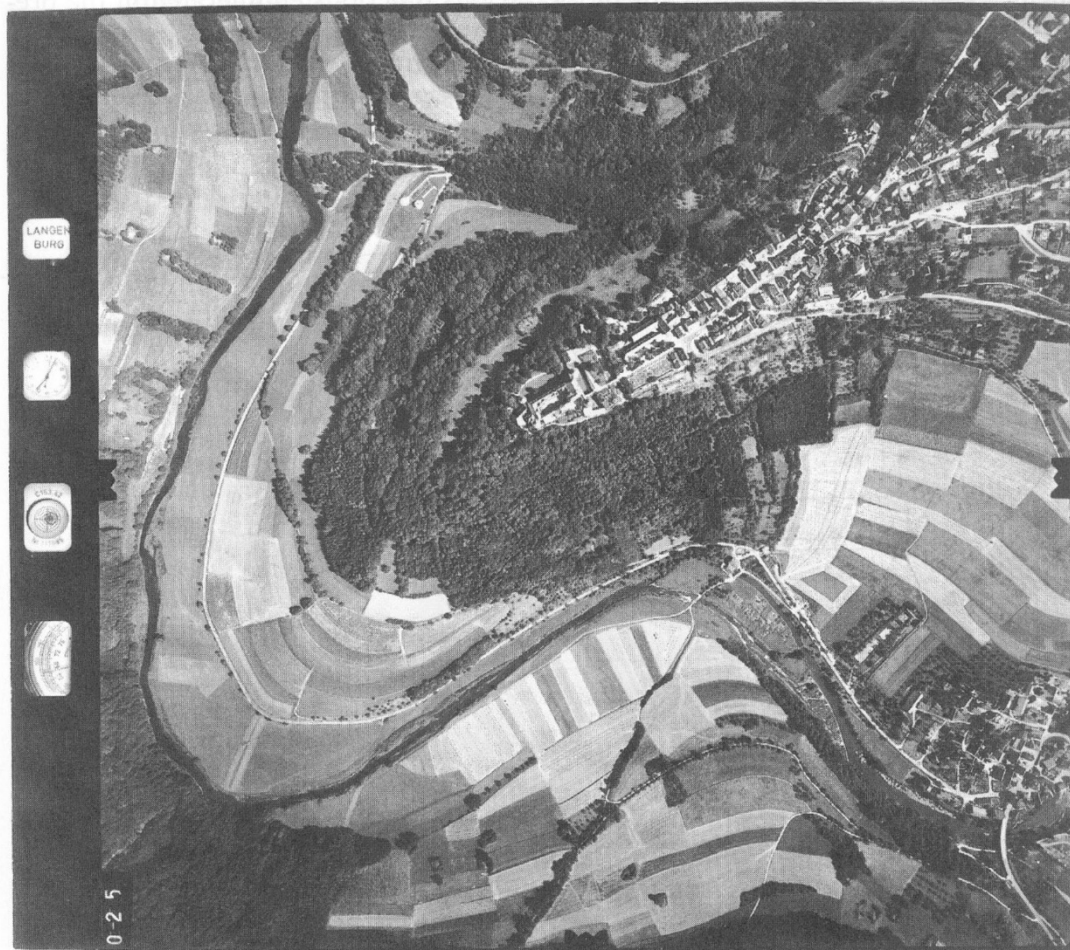
Figure 2.29 Vertical aerial photograph taken with a 230 \times 230 -mm precision mapping film camera showing Langenburg, Germany. Note the camera fiducial marks on each side of image. Data blocks (on left of image) record image identification, clock, level bubble, and altimeter. Frame number is recorded in lower left corner of image. Scale 1:13,200. (Courtesy Carl Zeiss.)
