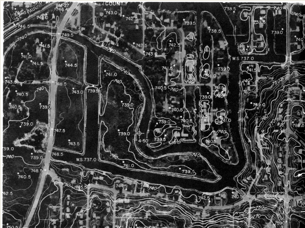
Portion of a 1 : 4800 topographic orthophotomap. Photography taken over the Fox Chain of Lakes, IL. (Courtesy Alster and Associates, Inc.)
