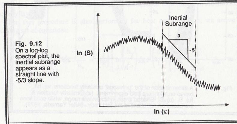
Fig. 9.12 On a log-log spectral plot, the inertial subrange appears as a straight line with  $-5/3$  slope.
