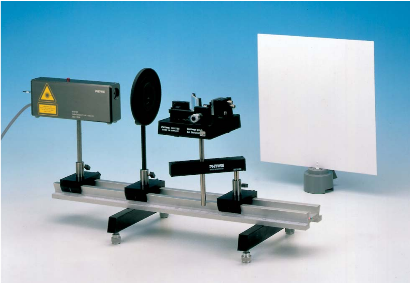
Fig. 1: Experimental set-up for measuring wavelengths with the Michelson interferometer.
