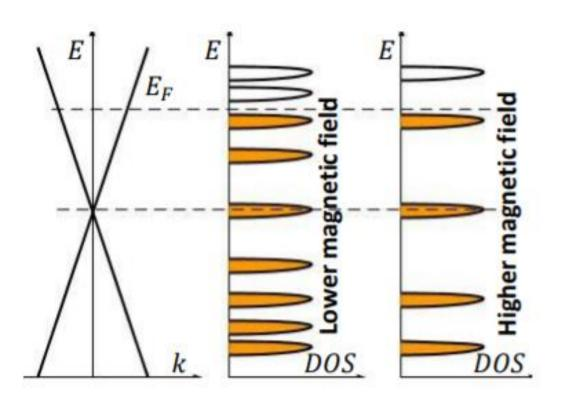
Lifshitz-Kosevich equation  $\Delta X(B,T) = A_0 A_T A_D A_S \left(\frac{B}{F}\right)^{\frac{1}{2}} \cos\left[2\pi \frac{F}{B} + \phi\right]$  $A_D = \exp\left(-2\pi^2 \left(\frac{k_B T_D}{\hbar\omega_C}\right)\right)$  $2\pi^2 \left(\frac{\kappa_B I}{\hbar\omega_C}\right)$  $A_S = \cos[\pi g m_e/2m_c]$
