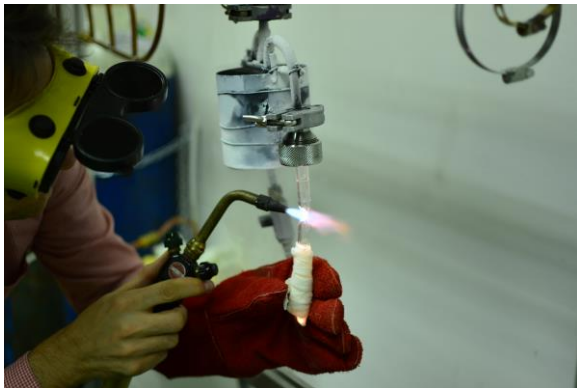
Sealing the quartz tube.
