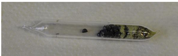
Material in vacuum sealed quartz ampoule (vacuum \sim 10^{-6} mbar)
