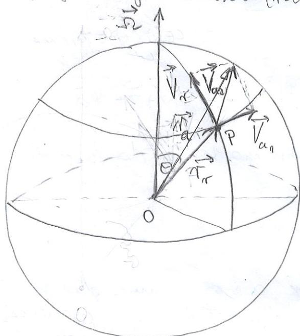
$$\vec{V}_{ar} = \frac{d\vec{r}_a}{dt} = \vec{V}_r + \vec{V}_{a_1} = \frac{d\vec{r}_r}{dt} + \vec{r}_r \times \vec{\omega} \Rightarrow \left| \frac{d\vec{r}_a}{dt} = \left( \frac{d\vec{r}_r}{dt} + \vec{r}_r \times \vec{\omega} \right) \vec{\omega} \right|$$
