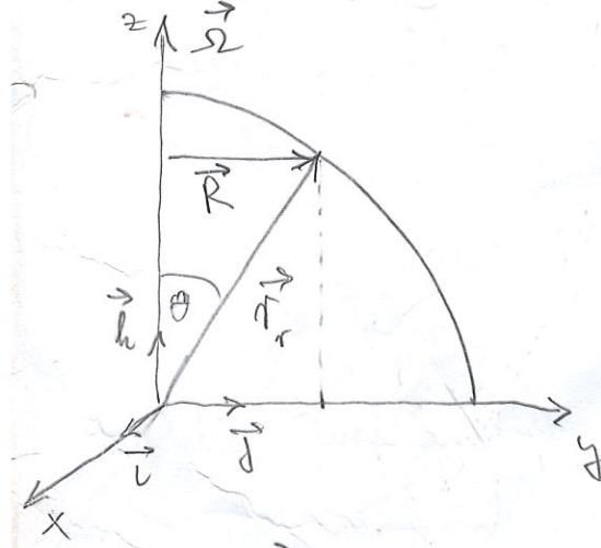
$$\begin{aligned} \vec{\omega} \times \vec{r}_a &= \vec{\omega} \hat{k} \times (\vec{r}_a \sin \theta \hat{j} + \vec{r}_a \cos \theta \hat{k}) = \\ &= -\vec{\omega} r_a \sin \theta \hat{i} \\ \vec{\omega} \times (\vec{\omega} \times \vec{r}_a) &= \vec{\omega} \hat{k} \times (-\vec{\omega} r_a \sin \theta \hat{i}) = \\ &= -\vec{\omega}^2 \vec{r}_a \sin \theta \hat{j} = \boxed{-\vec{\omega}^2 \vec{R}} \end{aligned}$$
