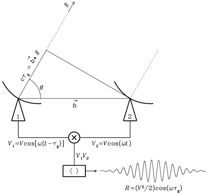
**Figure 1** A diagram of the components of a two-element interferometer. Vector  $\hat{s}$  points towards the target source,  $\vec{b}$  is the baseline. Output voltages  $V_1$  and  $V_2$  are multiplied and averaged by the correlator, creating a time-dependent interferometric fringe. (Source: NRAO)
