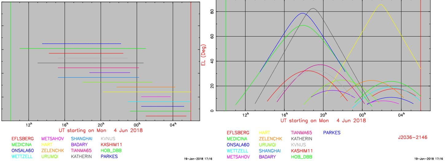
**Figure 6** SCHED output for uptime per telescope (left) and elevation vs. universal time (right) for target J2036-2146 on June 4th 2018. The 16 telescopes are listed below the image and in the text.
