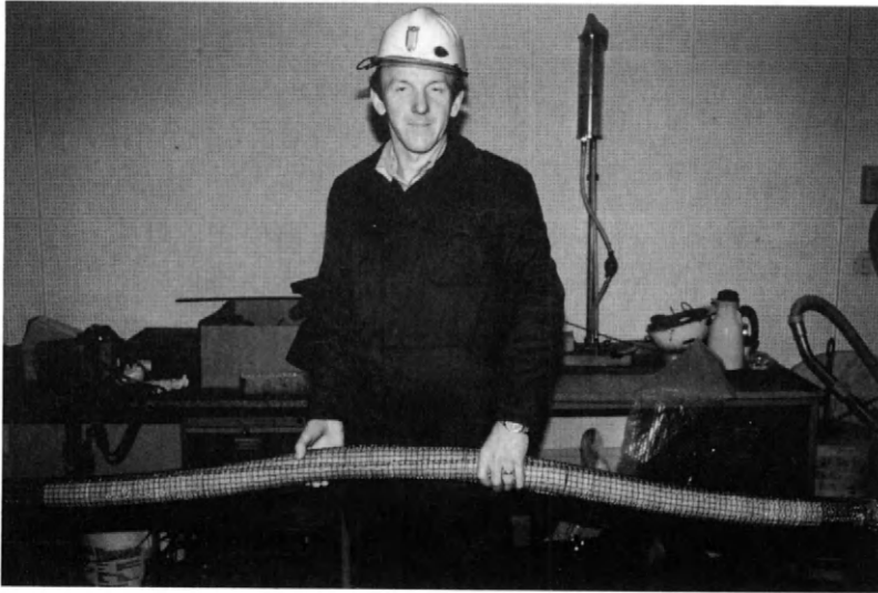
Figure 183 Upper: Insertion of 100 m long perforated pipe with highly compacted Na bentonite using hydraulic jack . Lower: Light but weak net-confined bentonite plug (NAGRA)
