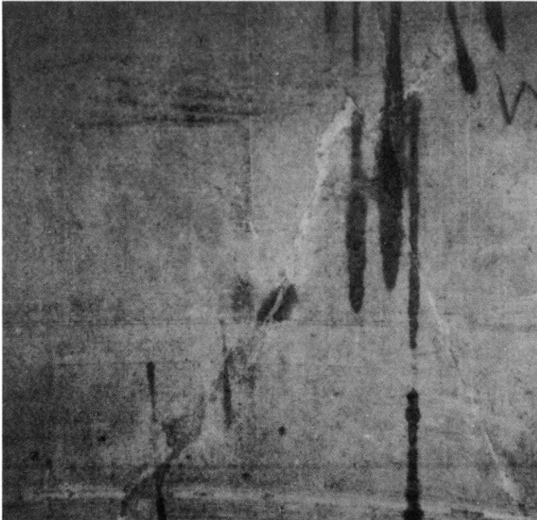
Figure 108 Photograph of the wall of one of the 0.78 m diameter core-drilled holes in the BMT experiment. Black blots are water flowing from fractures appearing white
