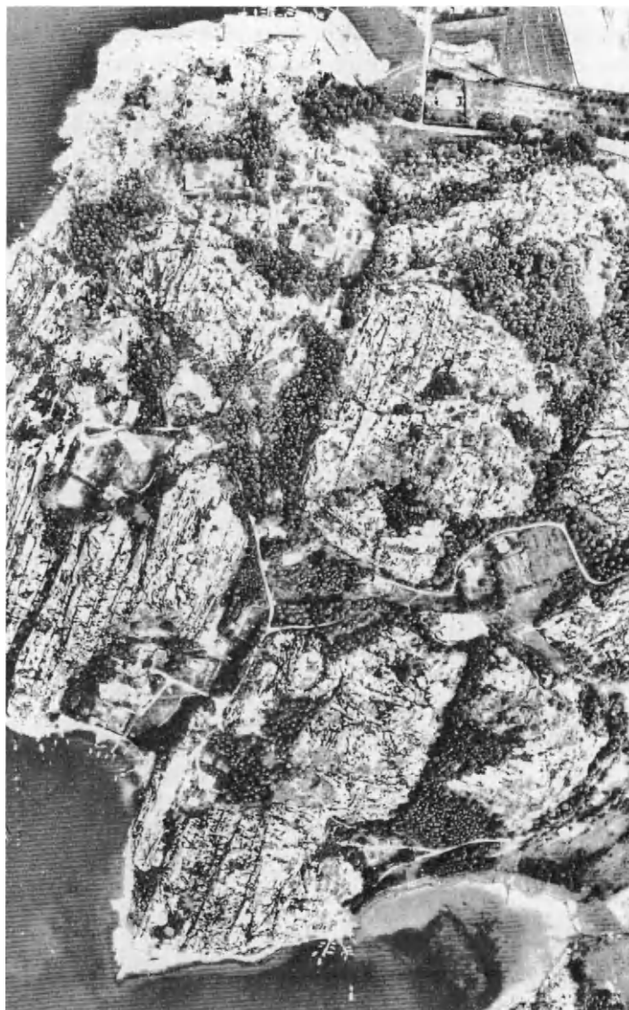
Figure 24 Aerial photo of granitic rock areas in Sweden. Notice the regular spacing and orientation of the large zones and the integrated “3rd order” zones. The width of the photo is about 700 m
