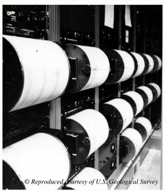
Seismic traces being recorded onto rotating paper charts (helicorders)
