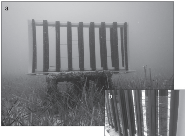
Fig. 1. Construction with plexiglass plates placed in meadow of Cymodocea nodosa seagrass (a), plexiglass plates placed in steel structure with plastic rails (b).
