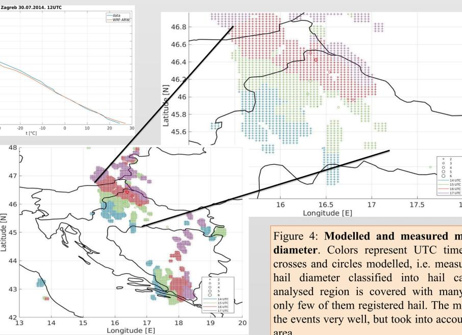
Figure 4: Modelled and measured maximum hail diameter. Colors represent UTC time, size of the crosses and circles modelled, i.e. measured maximum hail diameter classified into hail categories. The analysed region is covered with many hailpads but only few of them registered hail. The model simulated the events very well, but took into account too large an area.
