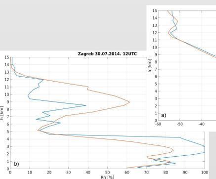
Figure 3: Measured and modelled vertical profiles of (a) temperature and (b) relative humidity at Zagreb Maksimir station at 12 UTC on 30 July 2014. They are strongly correlated for both parameters (also fig 7). The model slightly underestimates relative humidity in 1.5 to 4 km layer.
