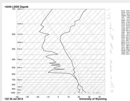
Figure 2: Sounding from Zagreb, Croatia at 30 July 2014 at 12 UTC. CAPE (CAPE = 857.7 J kg<sup>-1</sup>), LI index (LIFT = -2.65) and K Index (KINX = 37,60) indicate a strong potential for convective activity. Freezing level is found on 650 hPa and cloud base on 800 hPa. Strong dew point depression begins above 600 hPa.
