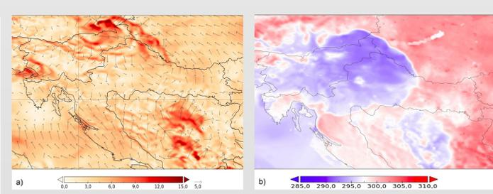
Figure 5: a) Modelled wind vectors (10 m a.g.l) and b) 2 m potential temperature on 30 July 2014 at 16 UTC at 3 km resolution. There were moderate to strong winds in the areas where hail had been predicted. The temperature field indicates cold pools which are associated with storm propagation.
