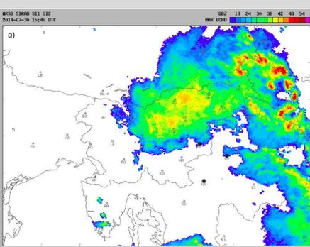
Figure 6: (a) Measured (15:40 UTC) and (b) modelled (16:00 UTC) maximum radar reflectivity (dBZ). In northern Croatia, spots with maximum radar reflectivity above 40 dBZ occur. We can link some of these areas with observed hail (fig 4). The modelled maximum radar reflectivity affects much larger area and has slightly higher values. It consequently predicts widespread hail.
